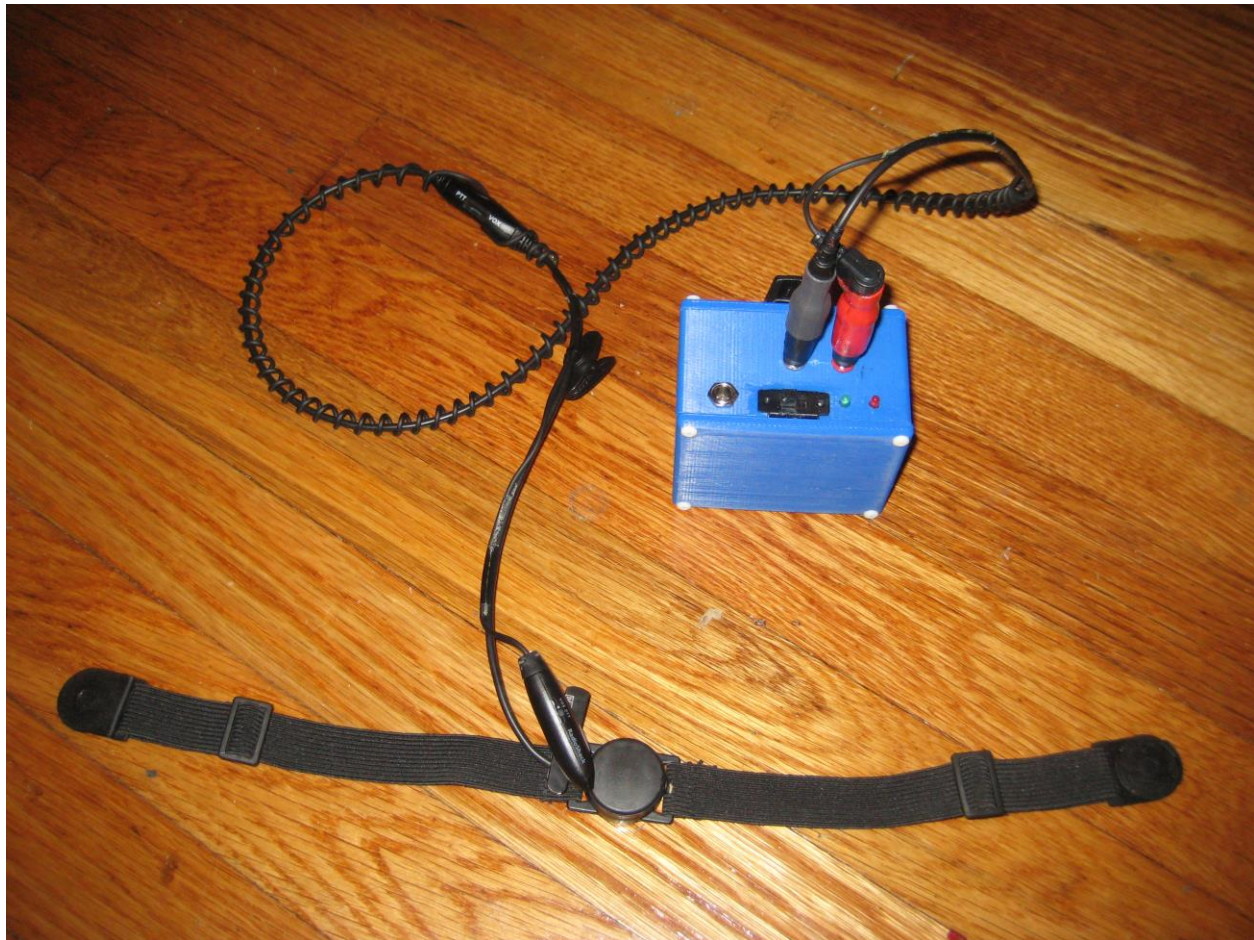
Fig. 7.18. The Voice Trainer. The microprocessor and circuitry are inside the enclosure in the top of the photograph, and the throat microphone and omnidirectional microphone are at the bottom.
