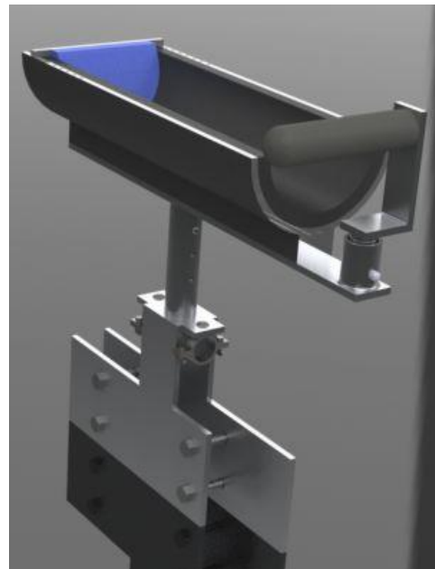
Fig. 10.14. Solid model of Midline Gait System attached to a walker.
