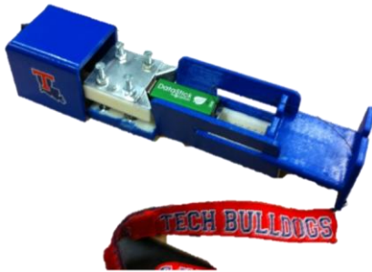
Fig. 8.13. Complete assembly of adaptive USB device.
