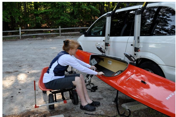
Fig. 19.7. The client moving lifting the kayak from the rack in its lowered position, and moving it to the cart for transporting it to the water.
