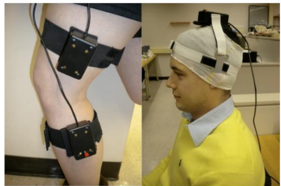
Fig. 12.25. As-built system being used to measure (left) knee flexion and (right) head tilt.
