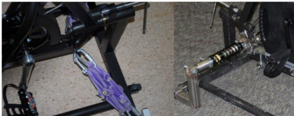
Fig. 12.13. Left: old tilt resistance mechanism. Right: new tilt resistance mechanism.
