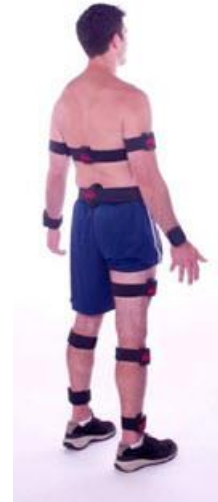
Fig. 22.3. Required sensor placements for the FAB system.
