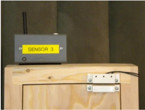
Fig. 8.15. Door sensor system showing magnetic switch on door and sensor with RF antenna.
