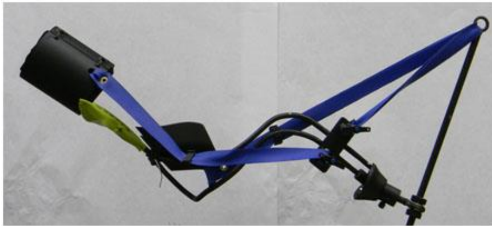
Fig. 10.12. Final Prototype of Mobile Arm Support.
