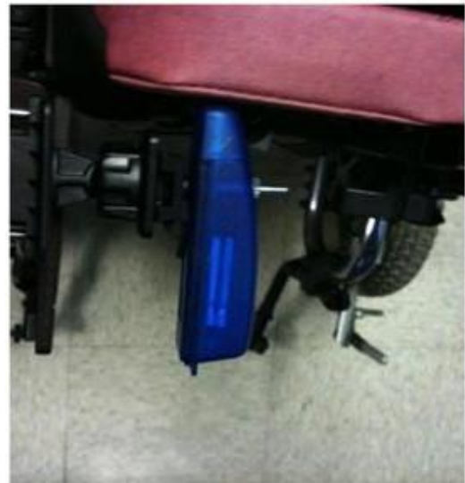
Fig. 16.5. Accelerometer mounted on wheelchair.
