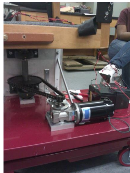
Fig.14. 8. Rotating Mechanism of Elevating Wheelchair Relocator.
