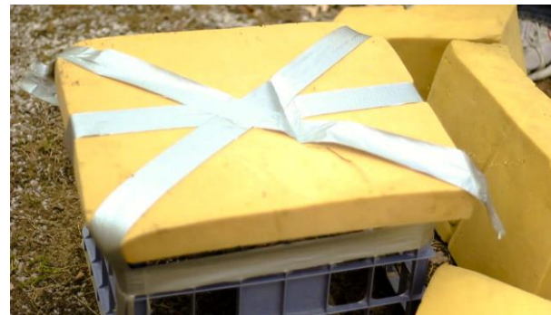
Fig. 10.2. Current transfer device consists of a milk crate with foam padding which acts as intermediate step.
