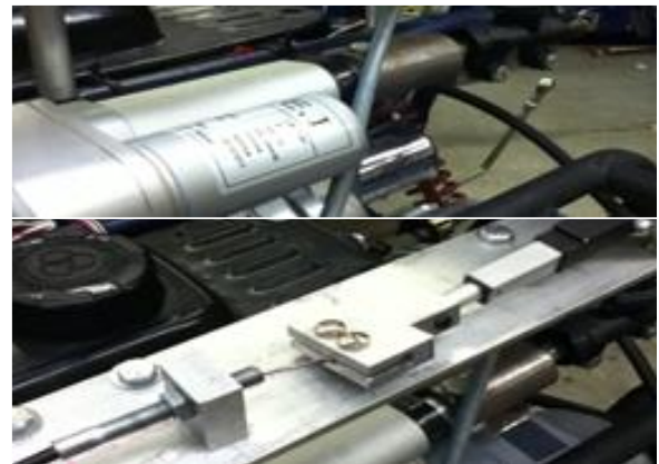
Fig. 17.2. Linear actuators for throttle (above) and braking (below).
