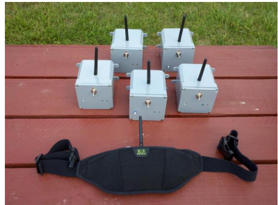
Fig. 19.8. The five radio beacons, with speakers mounted inside, that get mounted on weaving poles, and one radio detector that is worn by the user on a hip belt.
