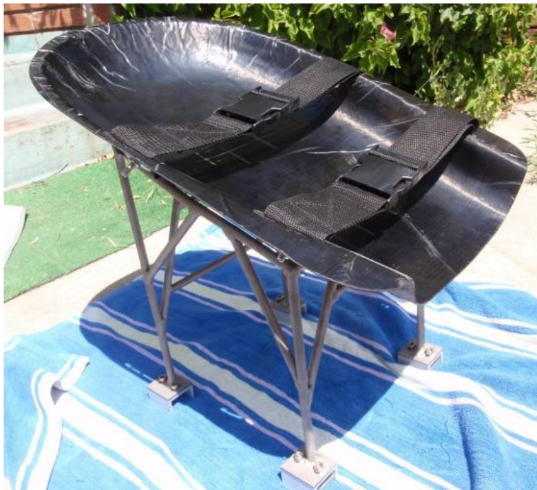
Fig. 6.20. Competition sit ski made from Titanium.
