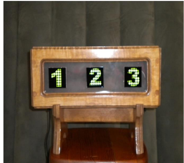
Fig. 8.19. Wall mounted unit showing LED matrices with corresponding door numbers
