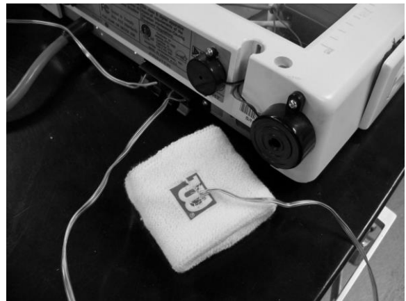
Fig. 21.2. Audio and physical alarms.
