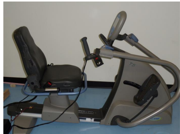
Fig.18.19. Position Adjustment Mechanism for NuStep Cross Trainer.
