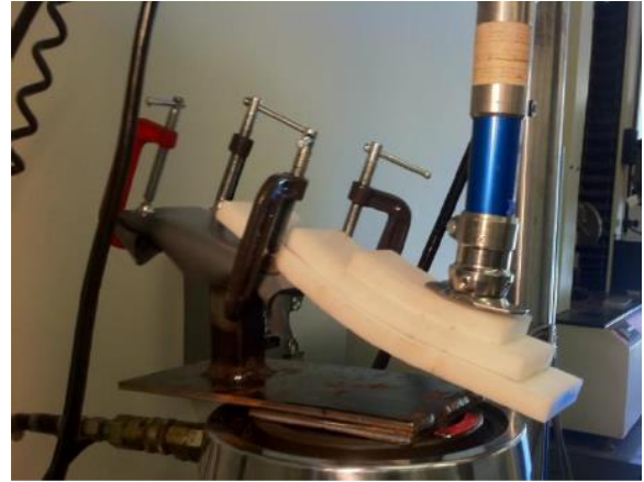
Fig. 6.42 PolyStack being tested on the Instron machine.
