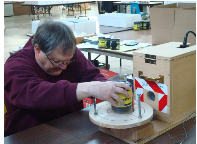
Fig. 7.11. An employee shrink wraps a nutritional supplement bottle using the EasyShrink.
