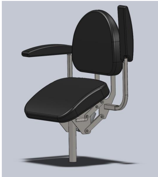
Fig. 20.6. SolidWorks Model Showing Tilting Motion of Seat, with the actuator fully retracted (top) and with the actuator fully extended (bottom).
